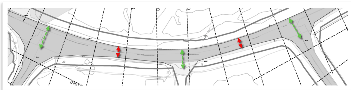
Figure 2.3 – Variance in Pavement Cross Section Likely to Create Confusion & Conflict
